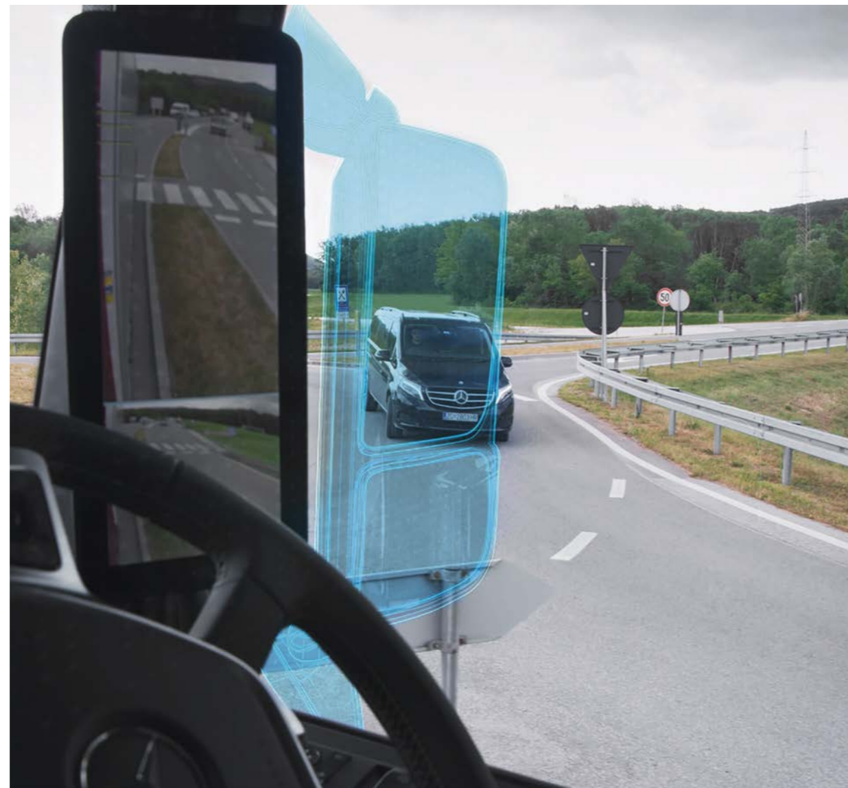
The new optionally available MirrorCam. The new system not only assists in saving fuel further still, but offers improved visibility to the rear and in the area of the A-pillar. Overseas model shown.
