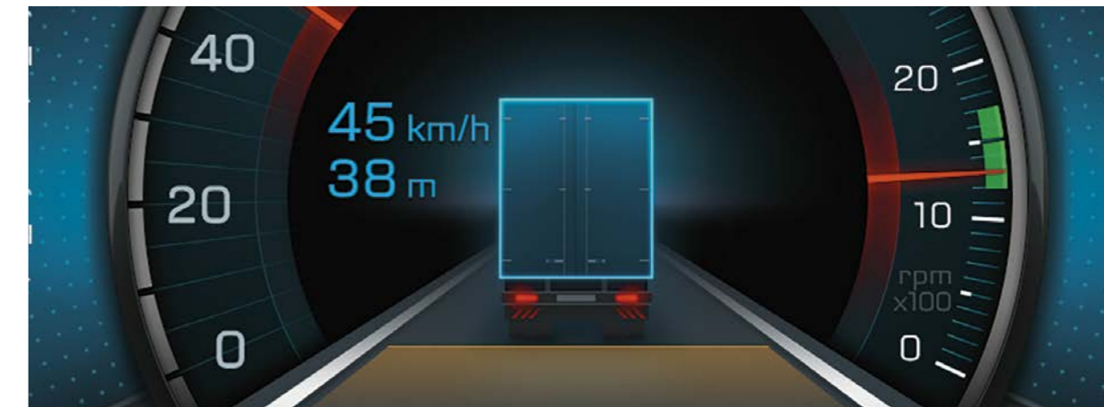
Proximity Control Assist 2) . This assistance system with stop-and-go function is on hand to support the driver in certain situations and can reduce the risk of rear-end collisions.
