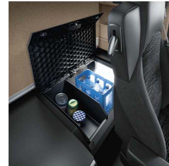
Exterior storage compartments. With a capacity of up to 420 l, the two storage compartments located under the bed in the L-Cabs can be accessed from both the inside and outside and offer a huge amount of storage space. Two adjustable storage trays are optionally available to allow better use to be made of the space.
