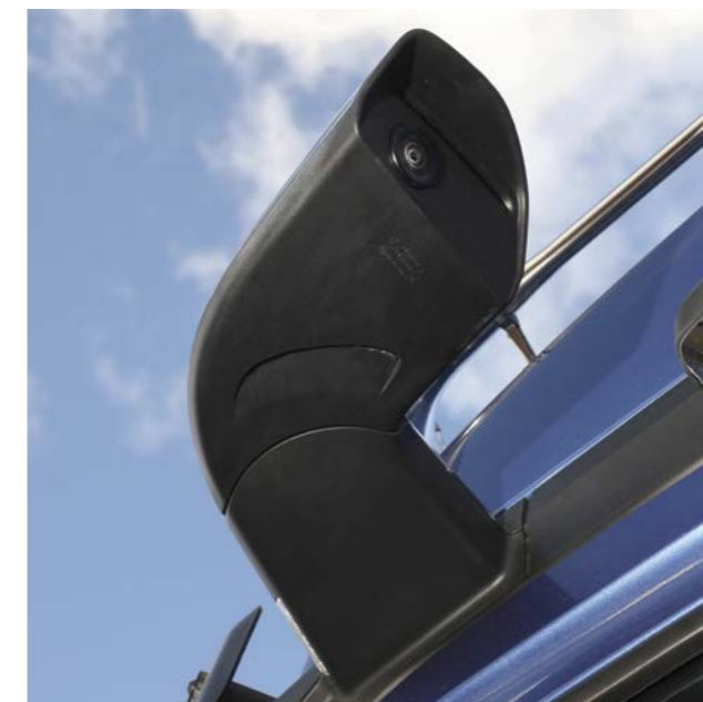
Aerodynamic eye-catcher. MirrorCam instead of conventional rear-view mirrors adds expressive visual and aerodynamic highlights to the new Actros.
