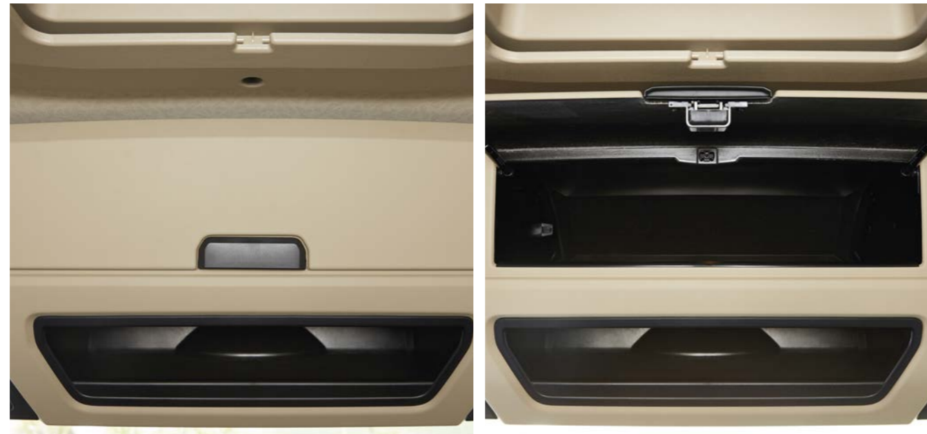
Storage compartments above the windscreen. As a result of the new, symmetrical arrangement of the storage compartments above the windscreen, the StreamSpace offers not only 161 l of storage capacity, but also excellent freedom of movement and headroom on the passenger's side. The upper storage compartments with hinged lids are illuminated on the inside, lined with slip-resistant felt and offer two drivers plenty of space.
