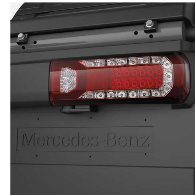
LED tail lamps. The new LED tail lamps send clear signals, especially the turn signal function, which features an outward-flowing light signal to indicate the direction.
