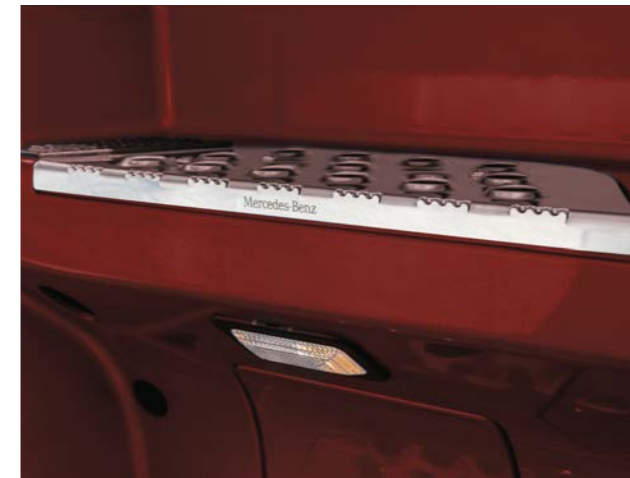
Stainless steel steps. Step by step: The custom-fit slip-minimising stainless steel steps for 2500 mm wide cabs not only provide a safer entry into your cab, but also enhance your vehicle's appearance 4) .
